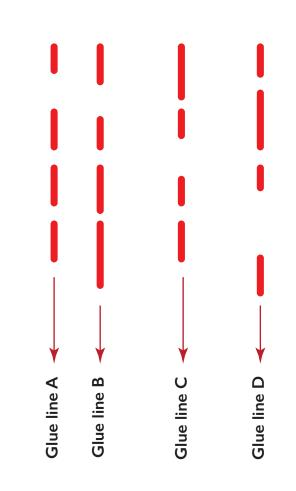
As long as the glue lines remain parallel you have full flexibility on the frequency of glue points along those lines. We are able to stop/start the glue points very accurately within +/- 0.5mm
